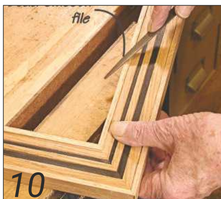
10 One or two strokes of this very fine file serve to trim the arris
