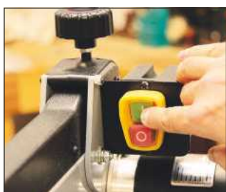
A rear-placed NVR provides the main power to the saw
