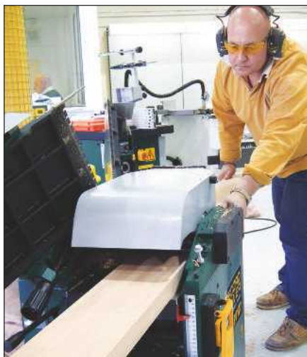
Planing the bow and twist from the bench-top's long beech boards involved removing 10mm of material
