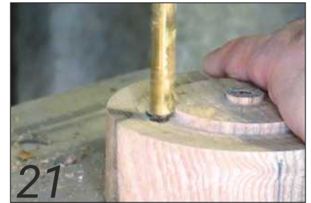
21 Drill an 8mm counterbore on the underside of the base about 6mm deep
