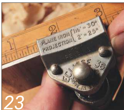
Setting the projection for the plane iron in the Eclipse 36
