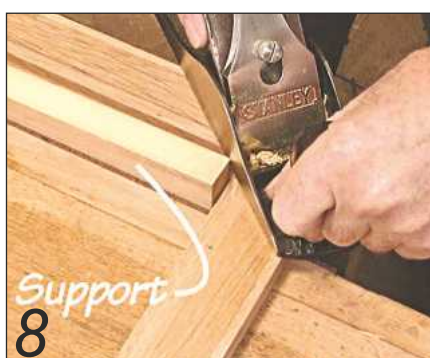
8 The support removes some of the risk in this tricky job
