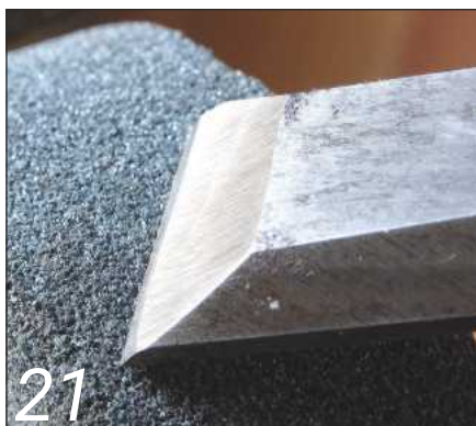
The hollow-ground primary bevel and 30° secondary bevel
