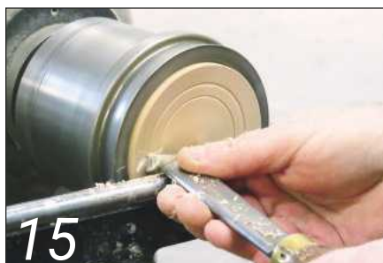
15 I cut a number of decorative beads on the top of the lid with a skew chisel
