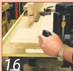
16 ... the end of the tops are grooved to take a ply tongue...
