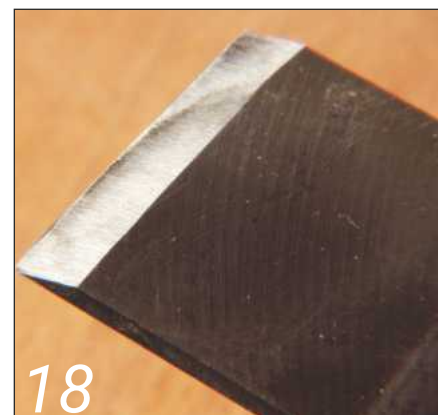
18 Hollow bevel developed on the grinding wheel
