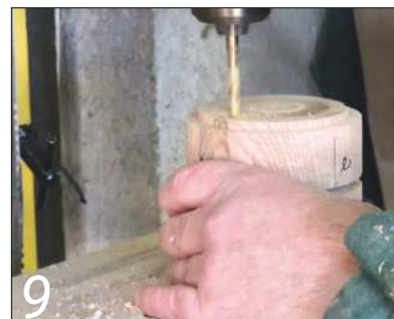
9 Back to the pillar drill to continue the hole in the middle tier
