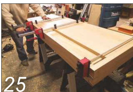
25 Once back on a horizontal surface, the top is clamped up and left to dry
