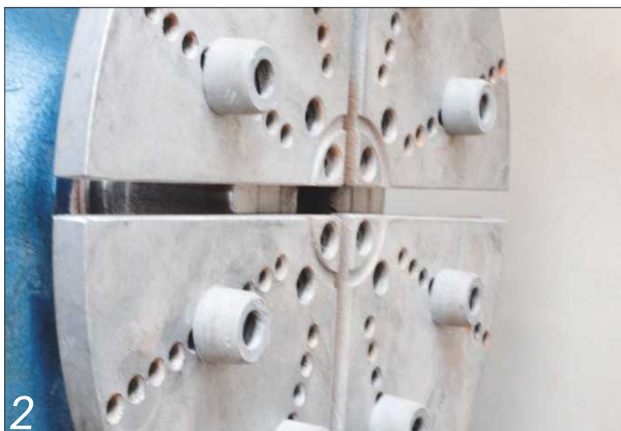
Adjustable button jaws are used for reverse chucking
