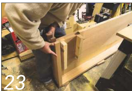
23 ... and with the front apron on the floor, the end aprons are set into place
