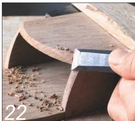
Freshly honed and paring a twisting bevel in end-grain
