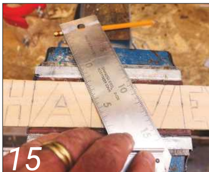
15 'Harvey' letters marked out. Set the angle for uniformity of slope
