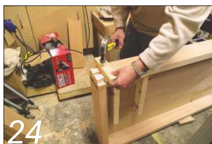
24 The final stage of assembly is to get the rear apron on and driven up
