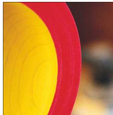
On unsealed maple a thin coat allows the grain to show through for a stained effect
