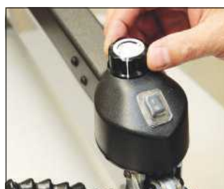
A small front-mounted rocker switch and variable-speed dial allow for fast control
