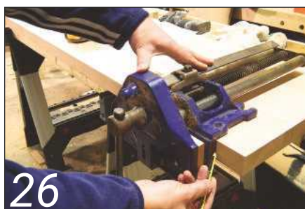
26 Mark the jaw width on the underside of the bench-top...
