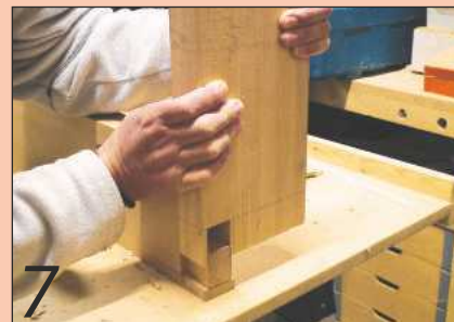
7 Using the joint as a template, the apron is marked up and cut
