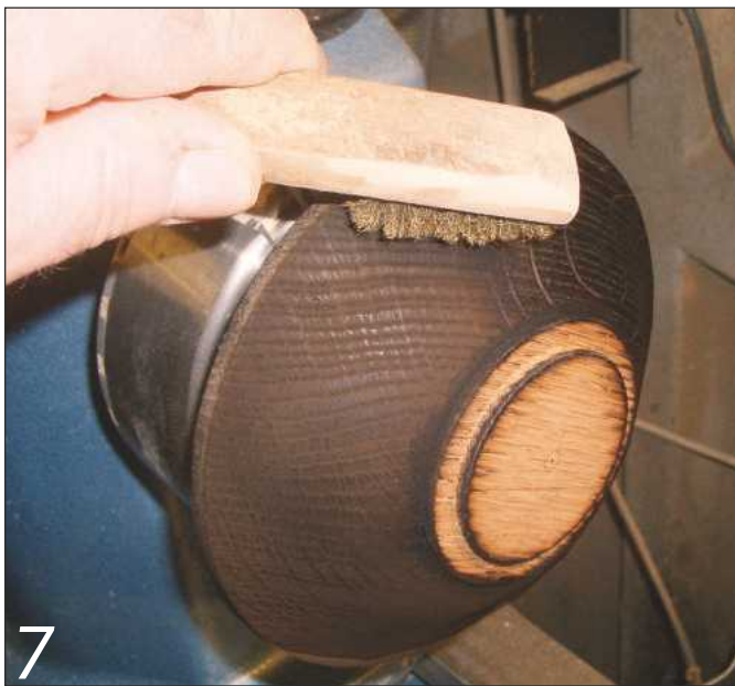
Wire-brushing removes loose charcoal and emphasises texture
