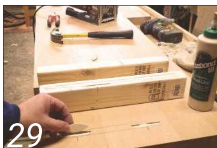
29 The packers are fitted with biscuits and glue before being drilled
