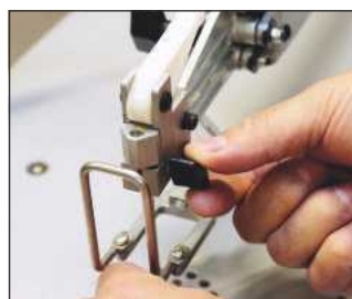
Blades are held with knobs so swapping for pierced work is quickly dealt with
