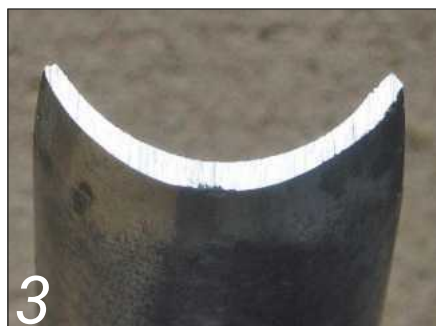
Next, the damaged end was ground back to a thick edge
