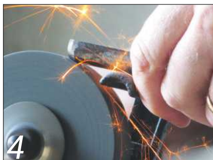
Shaping the bevel by pitching and rolling the blade
