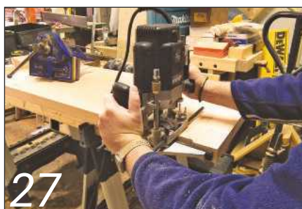
27 ... then rebate it to allow the rear jaw...
