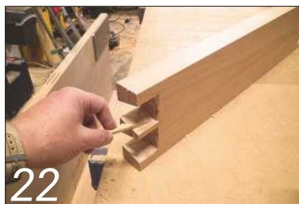
22 ... then the dovetails are glued up...
