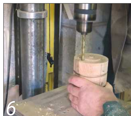
6 Drill a 6mm hole in the base, ensuring it is deep enough to mark the middle tier
