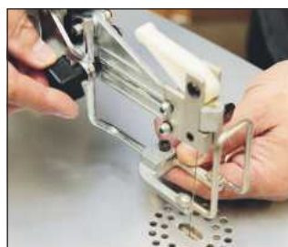
The hold down foot easily adjusts to minimise vibration and lifting as you work
