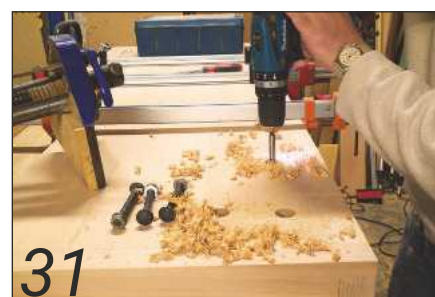
31 ... and the top drilled for the top-mounted coach bolts...
