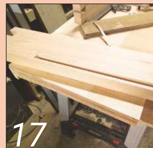
17 ... and a corresponding groove is worked into the end aprons
