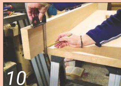
10 The aprons' length is set using the dry clamped boards to mark the shoulders...
