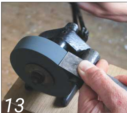
13 Finger positions while grinding
