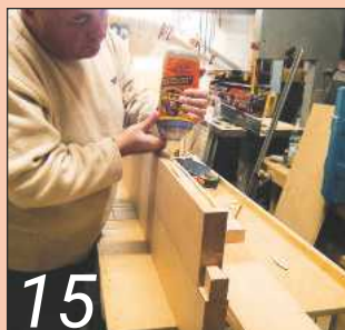
15 The main top boards are glued up, clamped and left to dry...
