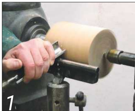
1 Mount the blank between centres and convert to a cylinder
