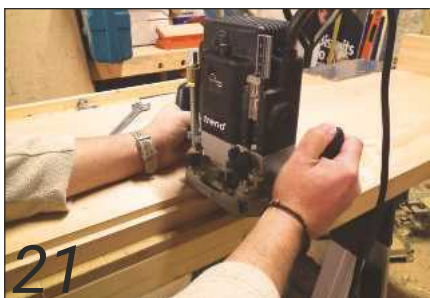
21 ... and on the underside a rebate was cut for the opposing edges of the tool well...
