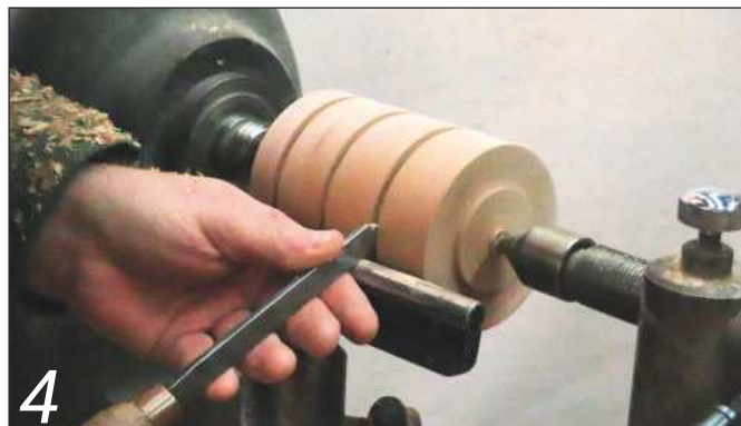
4 ... and make a 10mm deep parting cut at each mark
