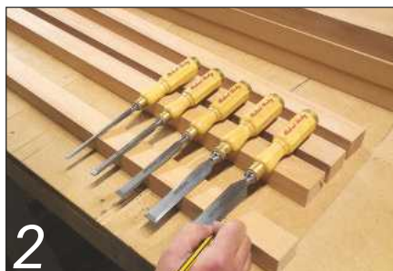
2 After ripping the board into four, the mortises are marked...
