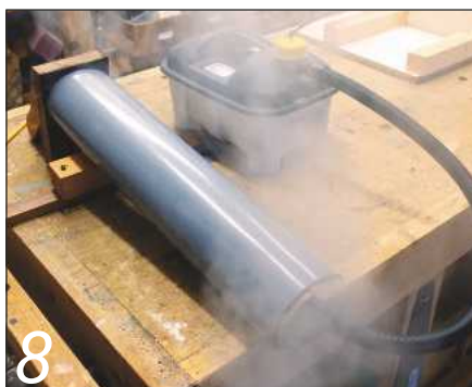
8 The drain pipe steamer
