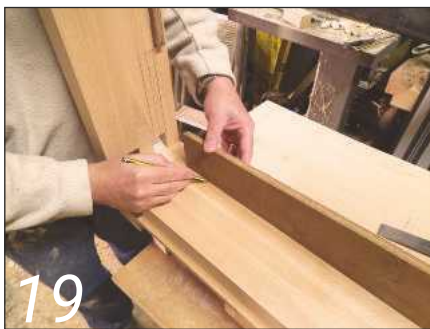
19 Using the well material as a gauge, the apron material was marked up
