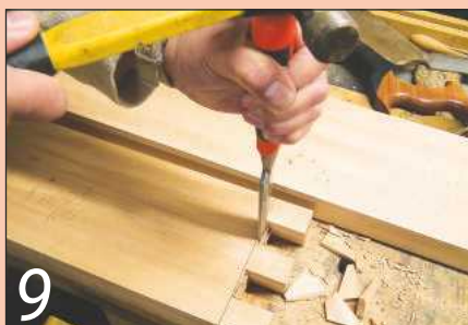
9 Drilling out the bulk of the waste made the chisel work substantially easier
