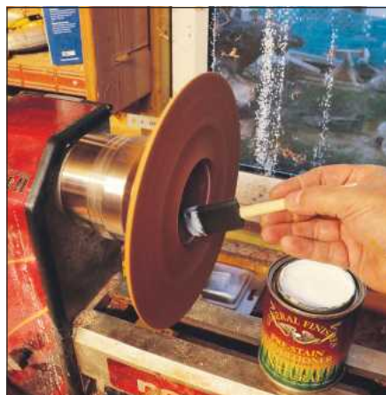
Sealing prevents stains drawing in and blotching on more porous timbers
