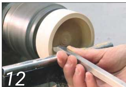
12 Use a scraper to square up the side of the hollow and flatten the bottom
