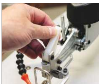
The quick-release tensioning cam allows faster blade alteration or swaps
