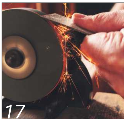
17 Back to the wheel for a block plane blade
