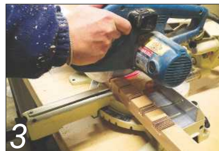
3 ... the slots cut on the chop saw, and the pieces glued back together
