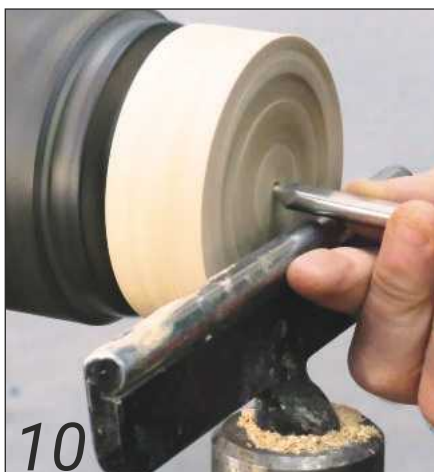
10 Hollow the base by first drilling a hole in the centre with a spindle gouge...
