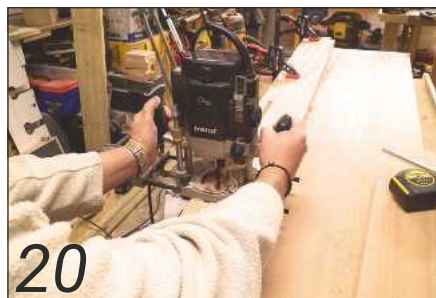
20 The groove was made in the rear and left-hand aprons cut using a router...
