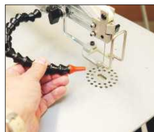
An articulated dust blower is built in to help keep the work area clear
