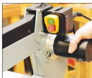
Releasing the screws and twisting the motor allows you to set up a pendulum movement
