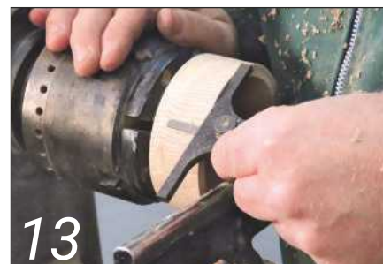
13 You can then check the depth of the hollow using a depth gauge
