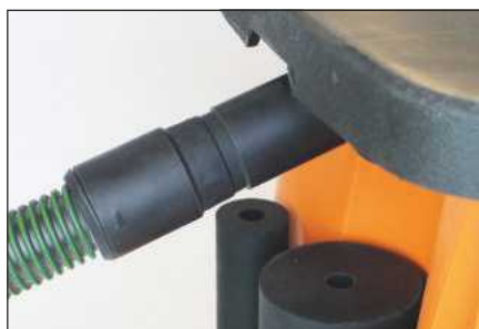
The (increasingly) standard Festool extraction hose fits the dust outlet perfectly
