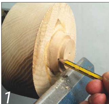
The face must be angled in the correct direction for the work to be properly supported
